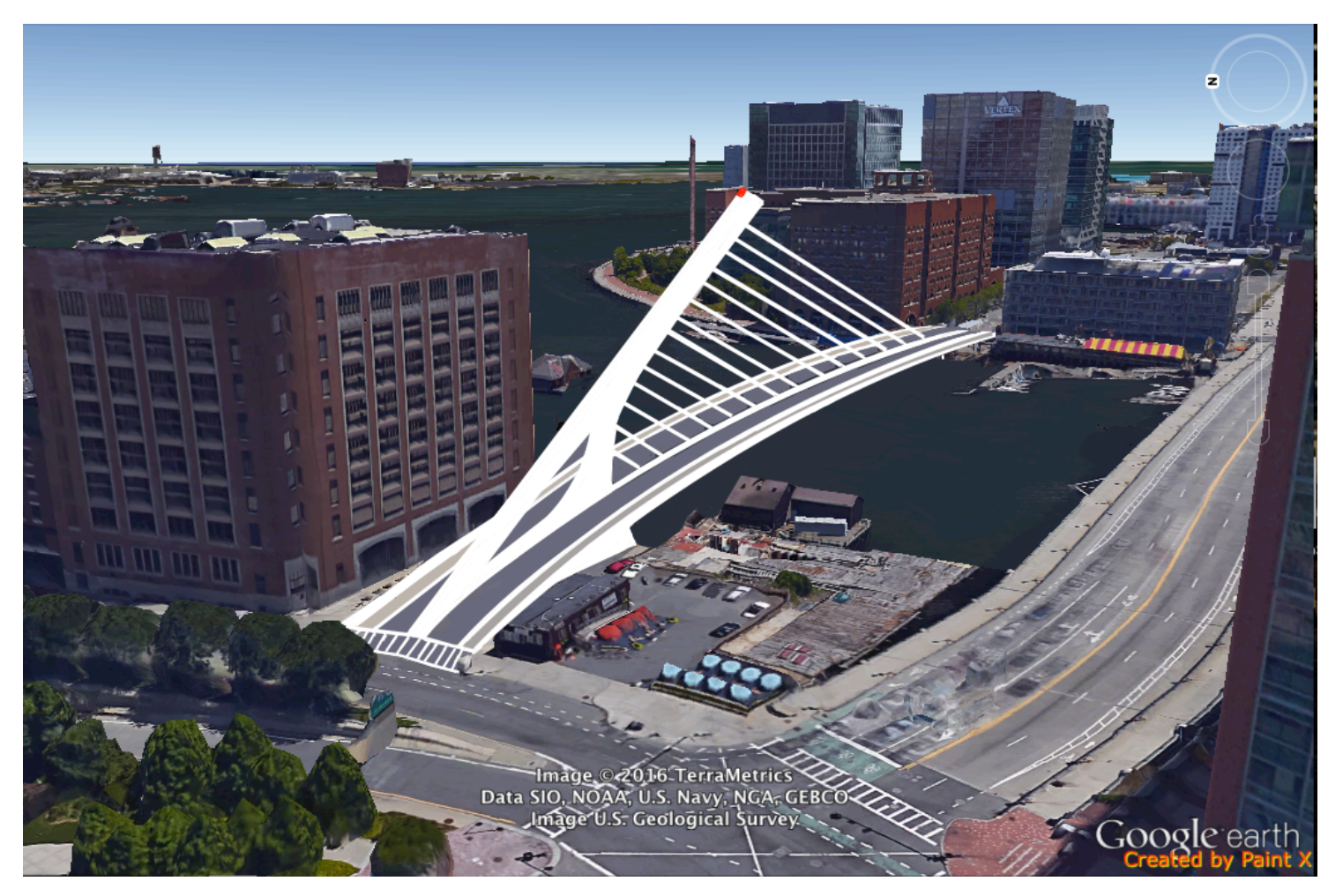
Bridge proposal with additional span cables in white.
